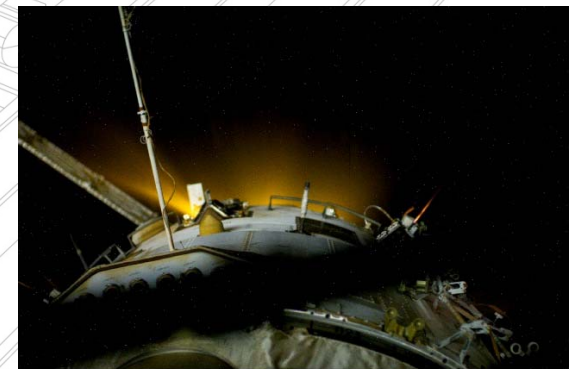
View of the first reboost burn by Progress M-47/10P. (from ISS Digital Imagery Management System)
